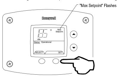
Step 3: Press the "UP" or "DOWN" buttons to change the maximum setpoint value. This will limit the maximum setpoint the user can select. Note: The maximum setpoint is approximately 180°F.
